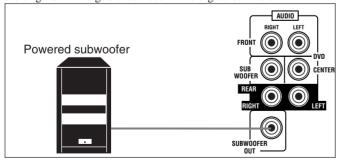
Connect the input jack of a powered subwoofer to the SUBWOOFER OUT jack on the rear panel, using a cable with RCA pin plugs (not supplied).
